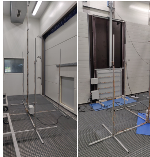
Figure 13: Hot and cold rooms sensor arrangements
