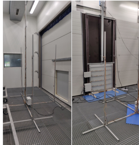
Figure 13: Hot and cold rooms sensor arrangements
