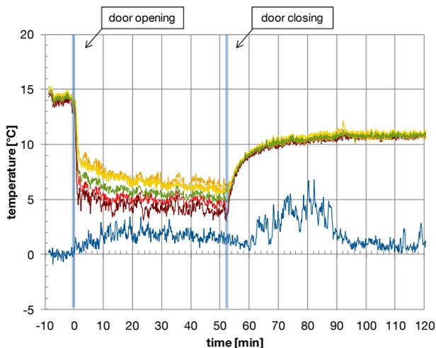
Figure 12: Temperature profile during door opening. The temperatures shown here refer to the measuring points in front (red lines) and rear (yellow lines) of the hall at a height of 1.4 m. Furthermore, an average interior temperature is calculated and shown as a green line. The measured outdoor temperature is represented as a blue line.
