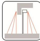
Laser technology is based on the principle of transit time measurement. In this case, a light pulse is emitted and the time until the reflection returns is measured.
