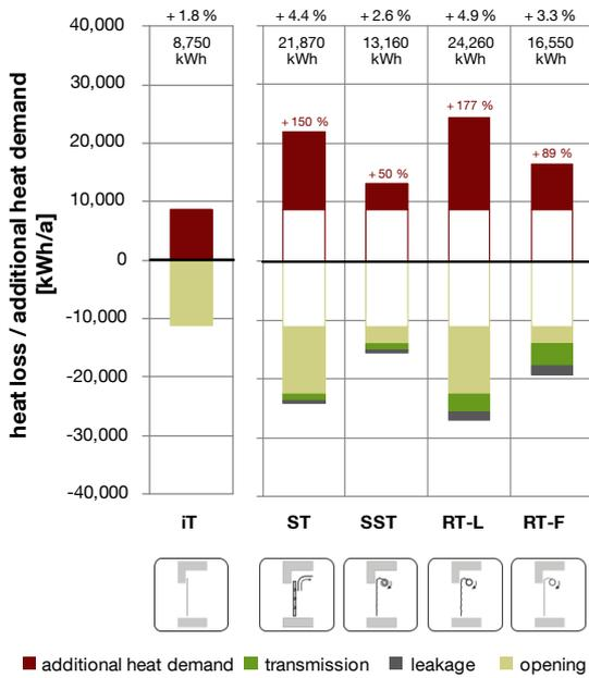
Figure 58: Additional heat demand and heat loss of each door in the scenario forklift traffic, 1-shift operation.
