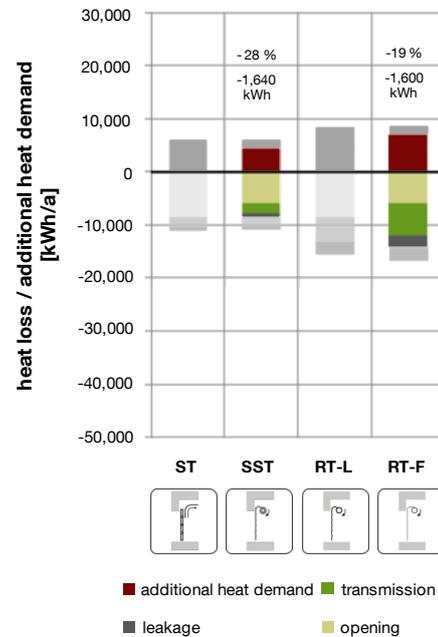
Figure 61: Reduction of the additional heat demand through frequent opening and closing of the door for the scenario truck loading / unloading, manufacturing building model.
