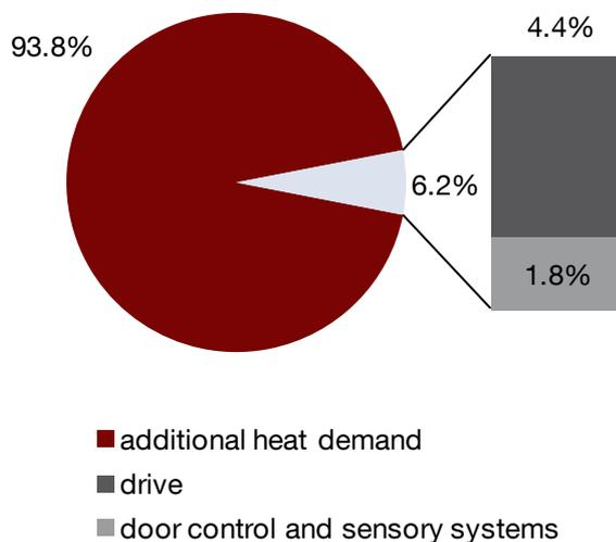
Figure 34: Comparison of energy consumption for heating, drive, door control and sensory systems. 2nd application: High-speed spiral door and scenario *regular forklift traffic*.
