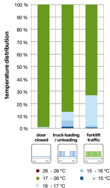
Figure 54: Temperature distribution of the scenarios of the *warehouse building model* at 1-shift operation in the "door zone" using the "ideal door" at a room height of 1.4 m during the operation time. Simulation time step: 30 s. Observation period: 1 year.
