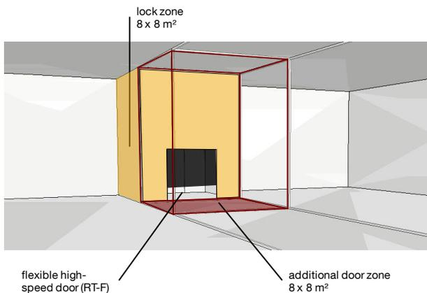
Figure 68: Interior view of the *manufacturing building model* in [IDA ICE 2012], showing the lock and the “additional door zone”.
