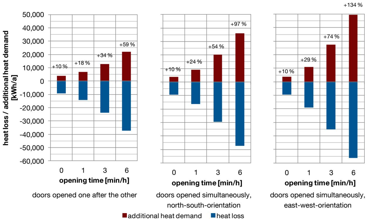
Figure 31: Additional heat demand and heat loss related to the respective building models without doors. Left diagram: doors opened one after the other. Middle diagram: doors opened simultaneously, north-south-orientation. Right diagram: doors opened simultaneously, east-west-orientation.
