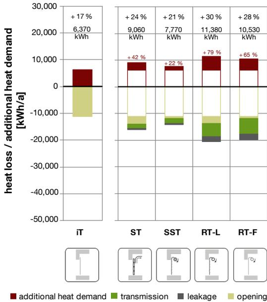
Figure 43: Additional heat demand and heat loss of each door in the scenario *mixed usage*.
