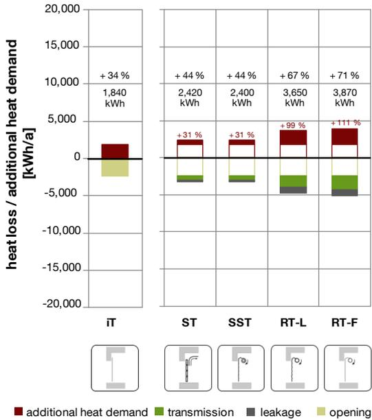
Figure 51: Additional heat demand and heat loss of each door in the scenario truck loading / unloading.
