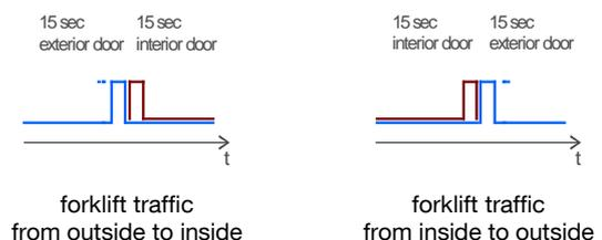
Figure 70: Lock function, regular alternating forklift traffic.
