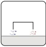
The influence of open doors on opposite sides of the building will be examined in this chapter as an example for the *manufacturing building model*. In this respect, an additional “door zone” with a second door is inserted into the 4-zone building model described in Chapter 5.2, see Figure 30.
