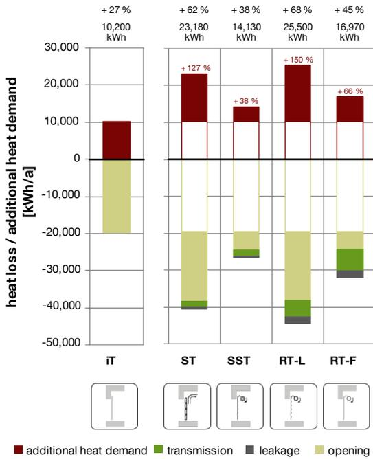
Figure 41: Additional heat demand and heat loss of each door in the scenario forklift traffic.
