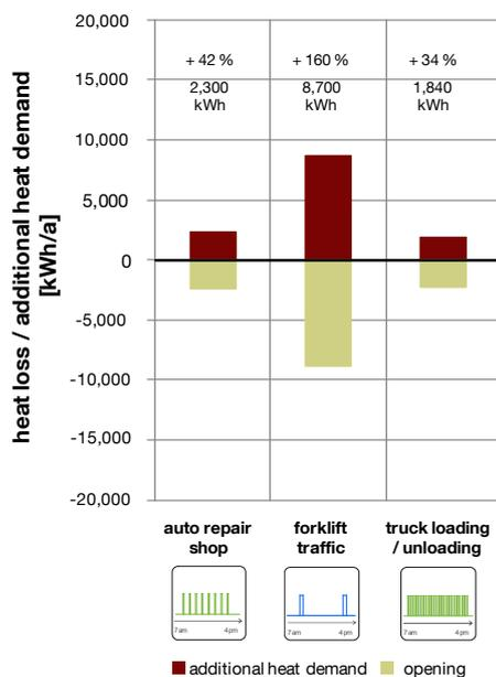
Figure 45: Comparison of the scenarios *auto repair shop*, *forklift traffic* and *truck loading / unloading* in terms of additional heat demand and heat loss for the "ideal door", workshop building model.
