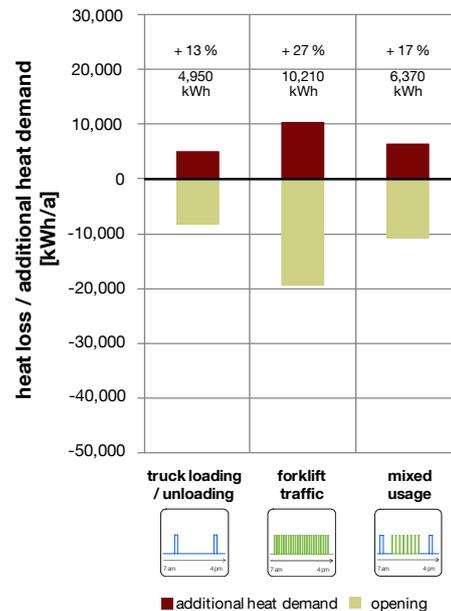
Figure 37: Comparison of the scenarios *truck loading / unloading*, *regular forklift traffic* and *mixed usage* in terms of additional heat demand and heat loss for the “ideal door”, *manufacturing building model*.
