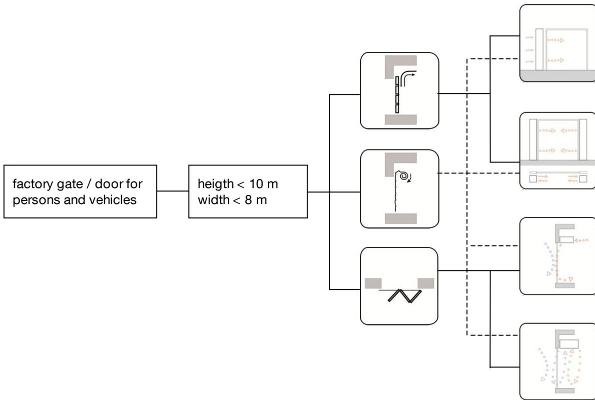
Figure 77: Overview of air curtains or air wall systems for different door types in accordance with [Frico 2013].
