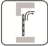
The most common used door type in industrial buildings is the sectional door [B+L 2010, 61]. It consists of several horizontally interconnected sections that result in the door leaf. The door is usually moved upwards when opening. In the upper opening position, the leaf can be moved upwards horizontally or folded [ASR A1.7, 6].
