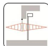
A radio control wirelessly transmits the signals by means of electromagnetic waves from a transmitter to a receiver. The receiver unit is placed at the door. An advantage of this manual control is
