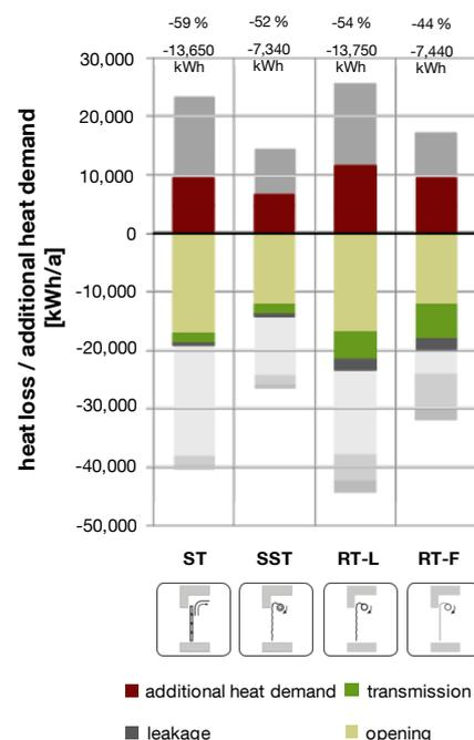
Figure 65: Reduction of additional heat demand through an object-size adapted opening, scenario *regular forklift traffic*, *manufacturing building model*.
