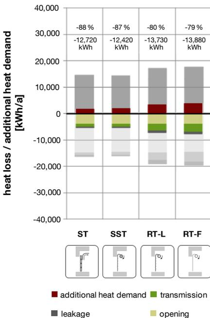
Figure 75: Reduction of additional heat demand through using a lock, scenario *truck loading / unloading*, warehouse building model, 1-shift operation.
