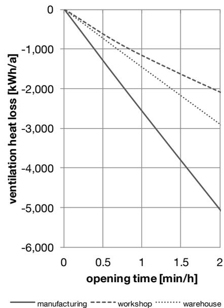
Figure 20: Ventilation heat loss in relation to opening time.
