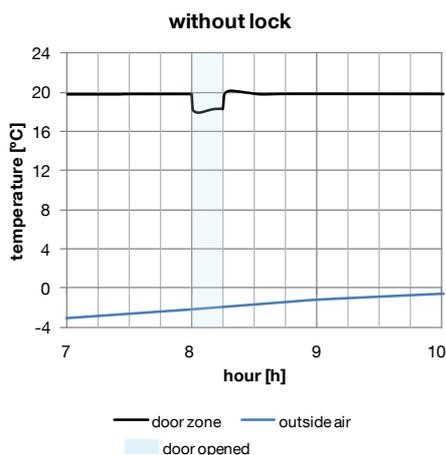
Figure 72: Outside temperature (blue line) and inside temperature at 1.4 m height (black line) in the door zone, *manufacturing building model* without lock, simulation period 01/23. 7 am – 10 am, scenario *truck loading / unloading*.
