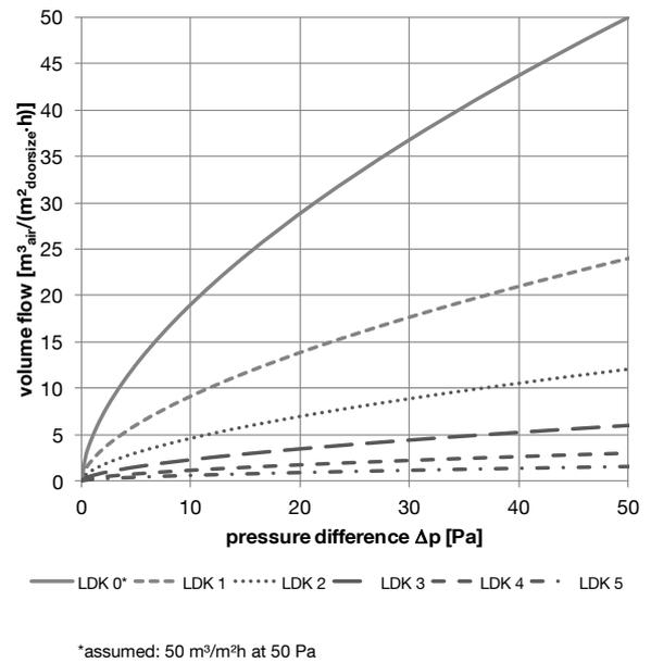
Figure 9: Relationship between pressure difference and air flow for different air permeability classes (LDK) according to [DIN EN 12426].
