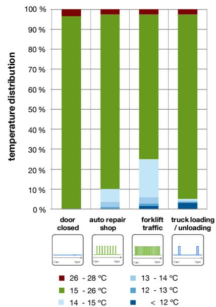
Figure 46: Temperature distribution of the scenarios of the *workshop building model* in the “door zone” using the “ideal door” at a room height of 1.4 m during the operation time. Simulation time step: 30 s. Observation period: 1 year.
