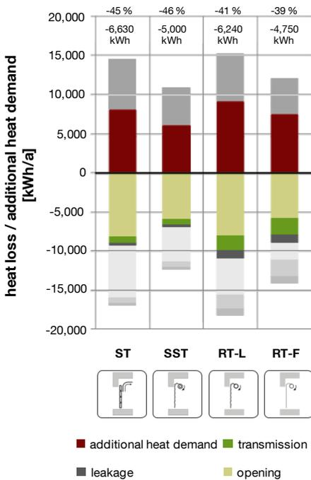
Figure 66: Reduction of additional heat demand through an object-size adapted opening, scenario regular forklift traffic, workshop building model.
