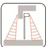
The radar detector sends microwaves at constant frequency in a defined area. When there is a movement caused by persons or vehicles in the detection area, waves with an altered frequency
