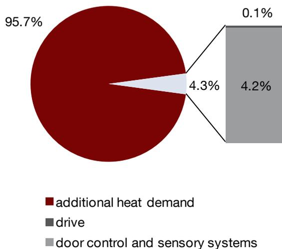
Figure 33: Comparison of energy consumption for heating, drive, door control and sensory systems. 1st application: sectional door and scenario *truck loading / unloading*.
