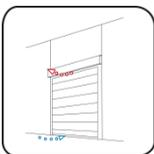
Doors like any multi-part constructions have joints (leakages), through which air can enter and escape. These leaks can vary depending on the door type. Therefore, the air permeability of doors
