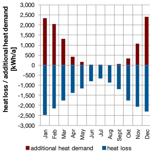
Figure 21: Heat loss through transmission, leakage and opening of the door and additional heat demand of one year with an average opening time of 6 min/h.
