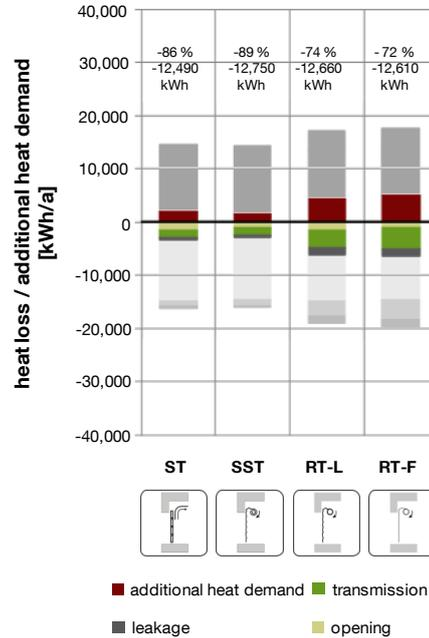
Figure 64: Reduction of the additional heat demand through truck loading / unloading in the building, warehouse building model, 1-shift operation.
