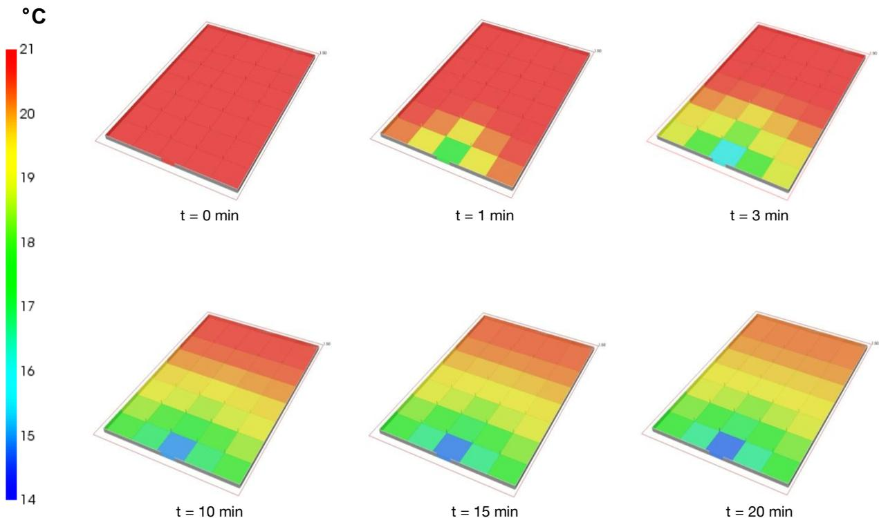
Figure 27: Simulated drop of interior temperature at opened door of the *manufacturing building model* on January 16 from 8:00 am to 8:20 am.
