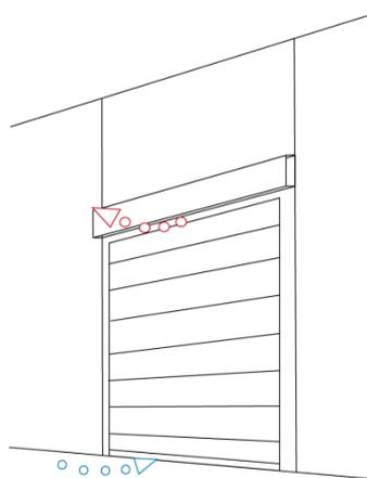
Figure 24: Heat loss caused by leakages.
