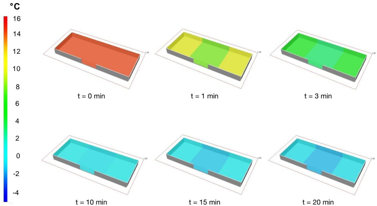
Figure 28: Simulated drop of interior temperature at opened door of the *workshop building model* on January 16 from 8:00 am to 8:20 am.
