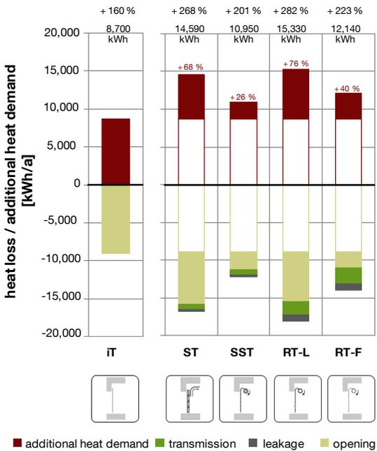
Figure 49: Additional heat demand and heat loss of each door in the scenario forklift traffic.
