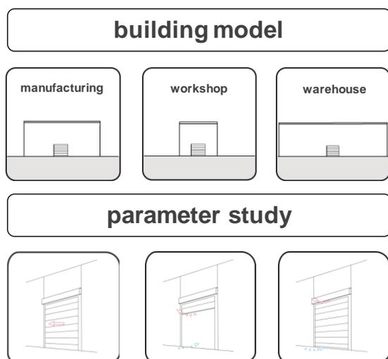
Figure 1: General approach of the parameter study: examination of different door-specific parameters, e.g. heat transition coefficient, opening duration and air permeability of the door.
