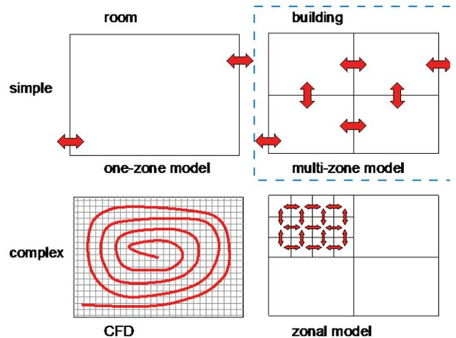
Figure 7: Different model types to calculate room air flows [Flieger et al. 2013].
