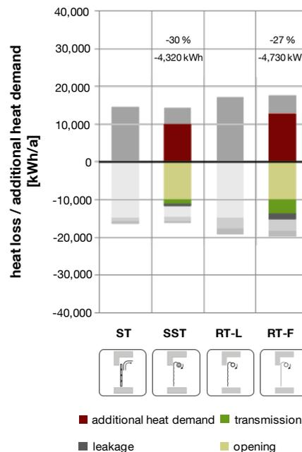
Figure 63: Reduction of the additional heat demand through frequent opening and closing of the door for the scenario *truck loading / unloading, warehouse building model* at 1-shift operation.
