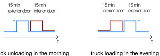
Figure 69: Lock function, truck unloading in the early morning (left), truck loading in the evening (right).
