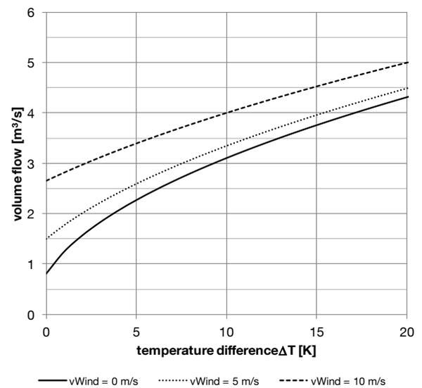
Figure 8: Air flows as a function of temperature difference and average wind speed at a square opening area of 16 m<sup>2</sup>.
