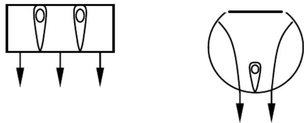
Figure 78: Comparison of conventional air outlet systems: fin (left) and nozzle (right) [Ketteniß 2007].
