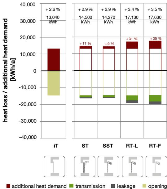
Figure 56: Additional heat demand and heat loss of each door in the scenario *truck loading / unloading*, 1-shift operation.
