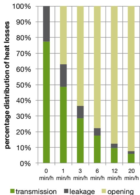
Figure 22: Percentage distribution of heat losses through the door by transmission, leakage and opening of the door in relation to the average opening time of the door as an example for the *manufacturing building model*.
