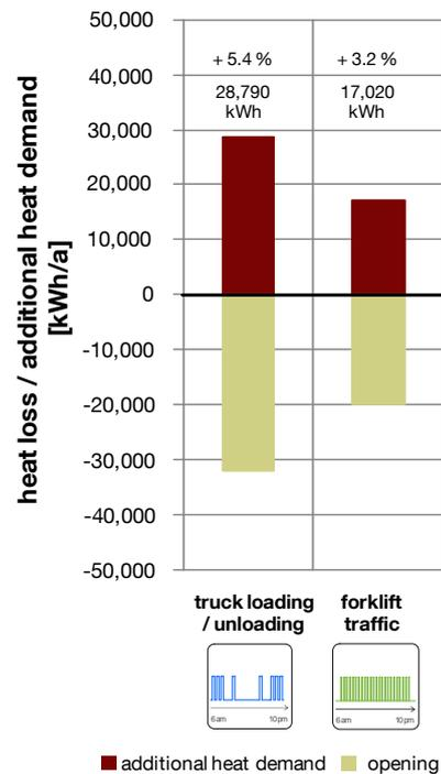
Figure 55: Comparison of the scenarios *truck loading / unloading* and *forklift traffic* in terms of additional heat demand and heat loss for the “ideal door”, *warehouse building model* at 2-shift operation.
