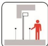
The dead man's control is a hold-to-run control, it requires a continuous operation for the opening and closing process and is done using a button.
