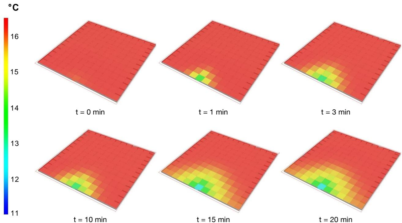
Figure 29: Simulated drop of interior temperature at opened door of the *warehouse building model* on January 16 from 8:00 am to 8:20 am.
