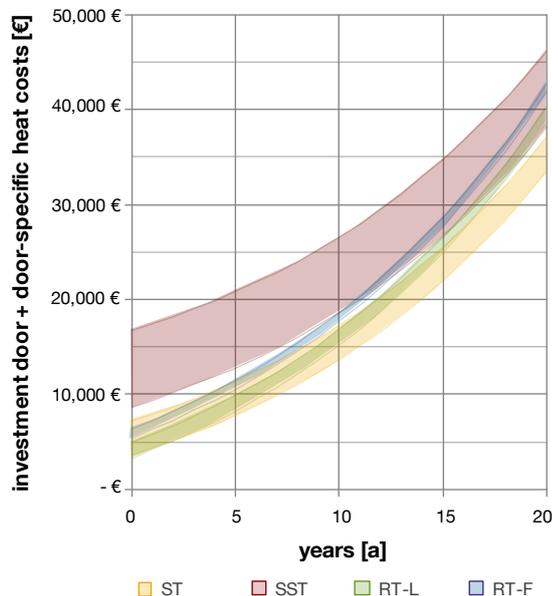
Figure 57: Door-specific investment and cumulated costs over 20 years in the scenario *truck loading / unloading*, 1-shift operation.
