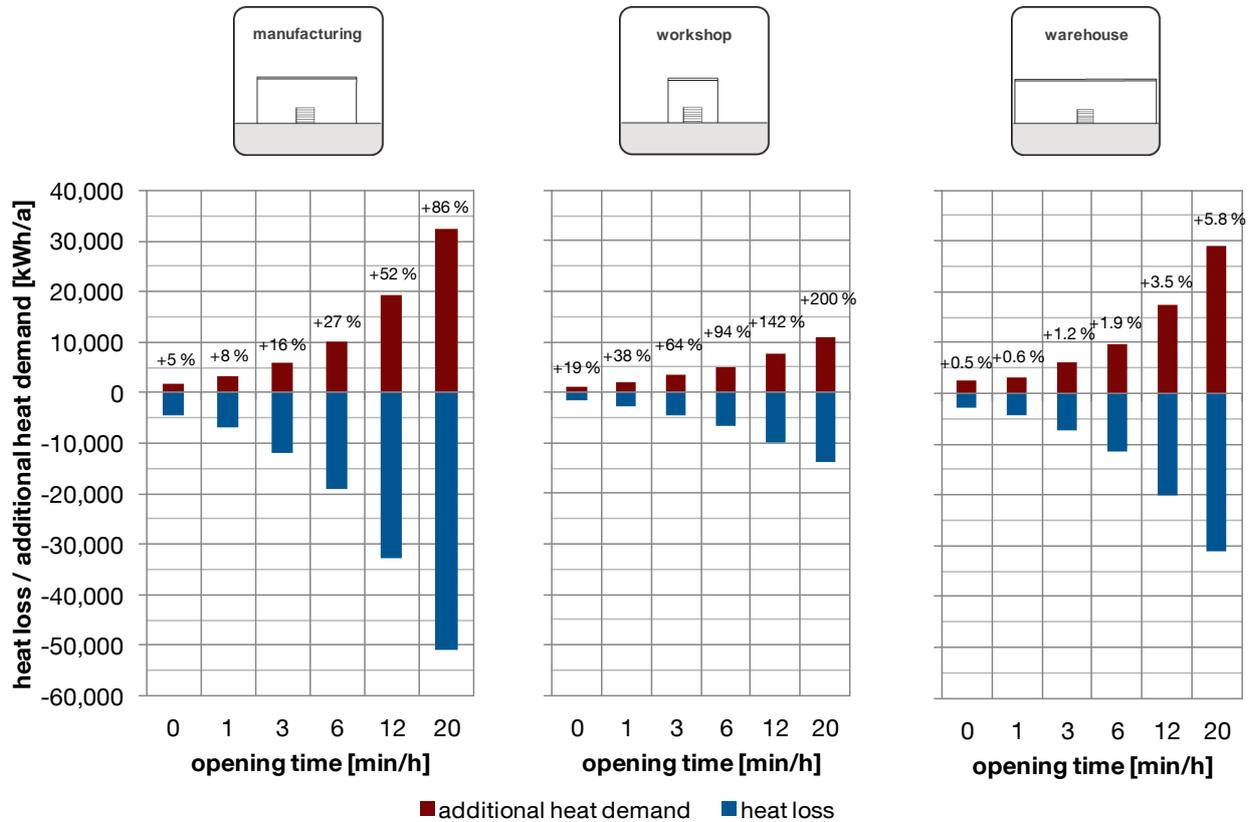
Figure 19: Heat loss through transmission, leakage and opening and additional heat demand related to the respective building models without doors for the building models manufacturing, workshop and warehouse.
