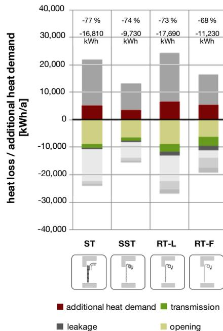
Figure 76: Reduction of additional heat demand through using a lock, scenario *regular forklift traffic*, warehouse building model, 1-shift operation.
