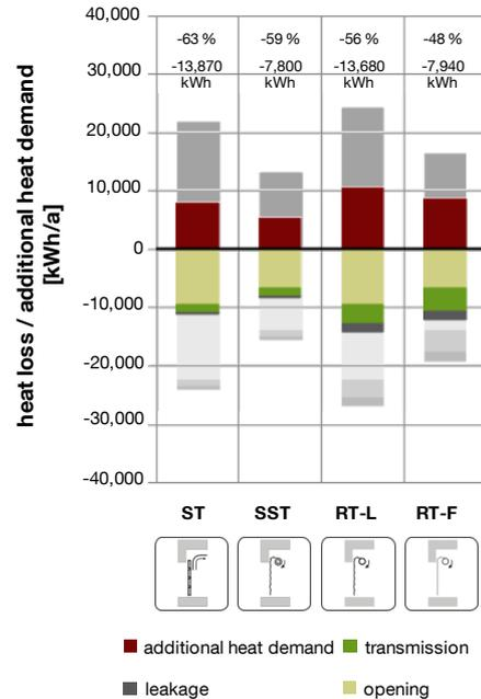
Figure 67: Reduction of additional heat demand through an object-size adapted opening, scenario regular forklift traffic, warehouse building model, 1-shift operation.
