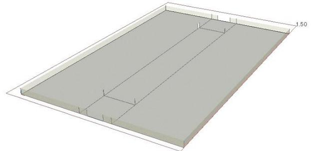
Figure 30: Section through the *manufacturing building model* in [IDA ICE 2012] showing the zoning and 2 doors on opposite sides.
