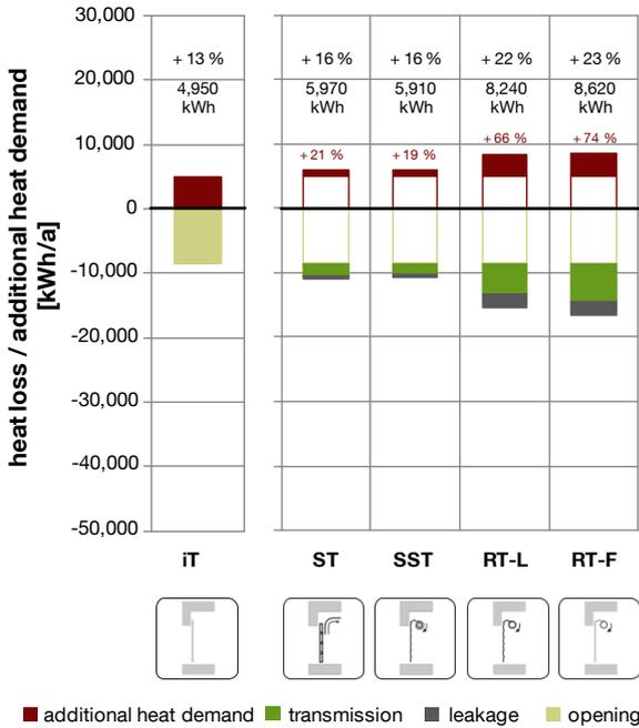
Figure 39: Additional heat demand and heat loss of each door in the scenario *truck loading / unloading*.
