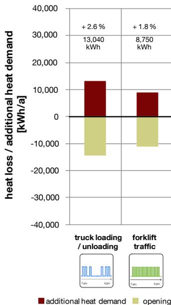
Figure 53: Comparison of the scenarios *truck loading / unloading* and *forklift traffic* in terms of additional heat demand and heat loss for the "ideal door", *warehouse building model* at 1-shift operation.
