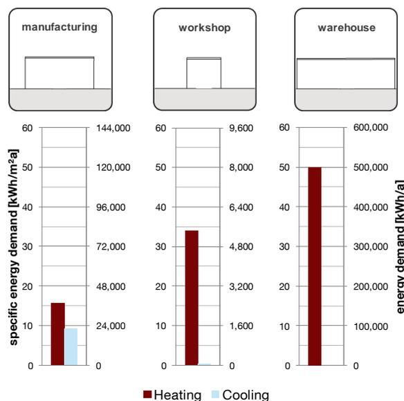
Figure 18: Specific and total energy demand for heating and cooling of the manufacturing, workshop and *warehouse building models* at 1-shift operation.
