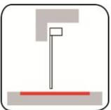
The induction loop uses the change of an electromagnetic field by metals for the registration of vehicles. So it is appropriate for automated door openings.
