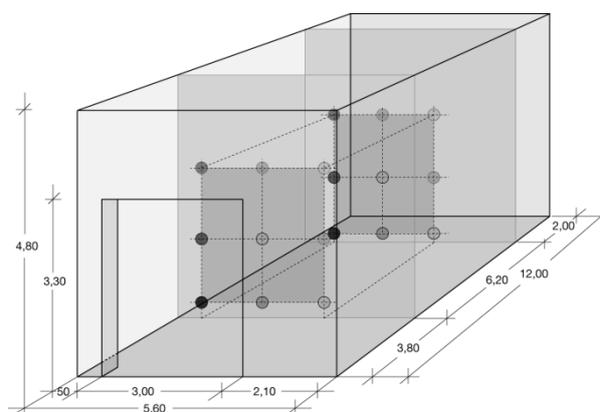
Figure 11: Experimental set-up for the temperature measurements with thermocouples.
