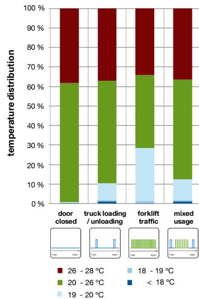
Figure 38: Temperature distribution of the scenarios of the *manufacturing building model* in the "door zone" using the "ideal door" at a room height of 1.4 m during the operation time. Simulation time step: 30 s. Observation period: 1 year.
