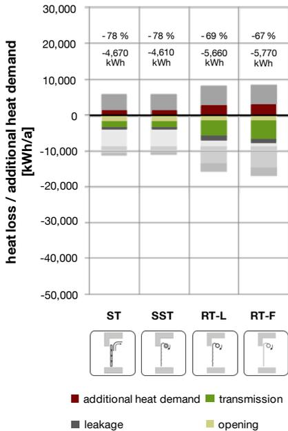
Figure 71: Reduction of additional heat demand through using a lock, scenario *truck loading / unloading*, *manufacturing building model*.
