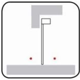
The photocell is an electronic optical system, which detects the interruption of a light beam and comprises a light beam source (transmitter) and a sensor (receiver).
