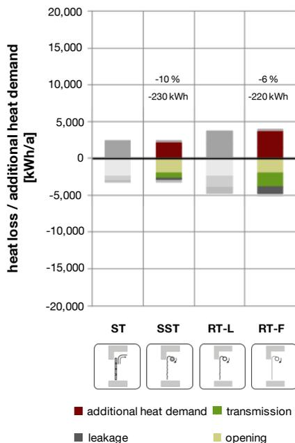
Figure 62: Reduction of the additional heat demand through frequent opening and closing of the door for the scenario *truck loading / unloading, workshop building model*.
