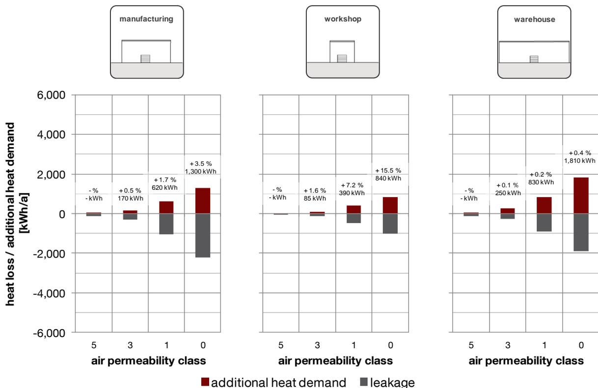
Figure 26: Variation of the air permeability of the door.
