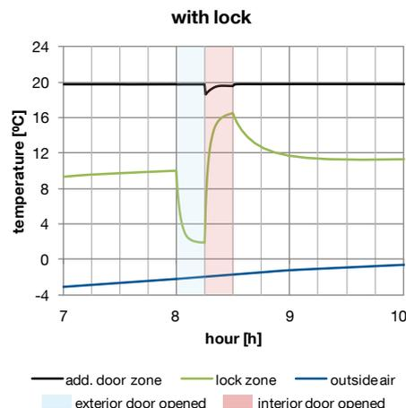
Figure 73: Outside temperature (blue line), inside temperature at 1.4 m height of the additional door zone (black line) and inside temperature at 1.4 m height of the lock zone (green), *manufacturing building model* with lock, simulation period 01/23 7 am – 10 am, scenario *truck loading / unloading*.
