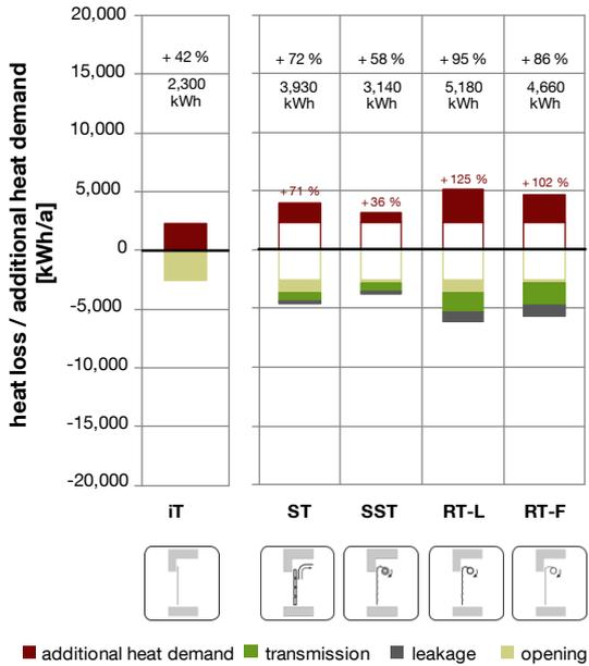
Figure 47: Additional heat demand and heat loss of each door in the scenario *auto repair shop*.
