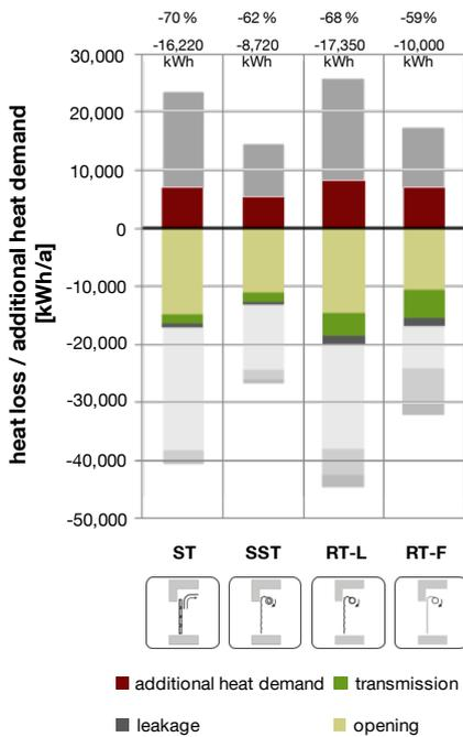
Figure 74: Reduction of additional heat demand through using a lock, scenario forklift traffic, *manufacturing building model*.
